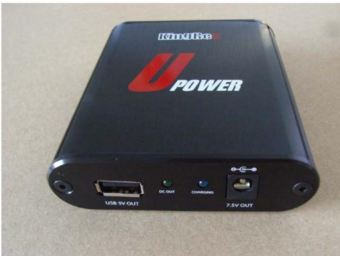
7.5V OUT: DC 7.5V output connector for Kingrex 7.5V series devices exclusively. For example: UC192, UD384 and...
