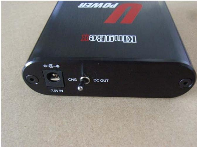
7.5V IN: Power input connector for your UPower charger (DC7.5V)
